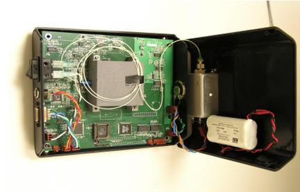
Figure 2. Battery-powered TDLAS sensor in a 6" x 7" x 1.5" package, consumes < 1W for continuous operation at a 10 Hz data reporting rate, and provides digital interfaces.
