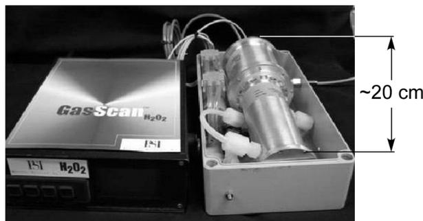
Figure 5. TDLAS analyzer assembly.
